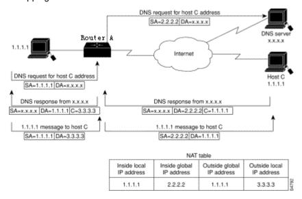
Figure 2-3 Network Condition Where NAT Translates Overlapping Addresses
